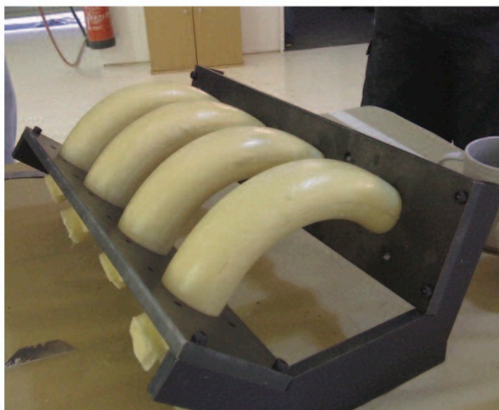
LEFT & BELOW The foam cores for the inlet manifold fitted to the jig prior to laying up, above. The finished product, below, includes bell mouths made using the same technique
