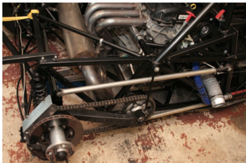
ABOVE & BELOW The CAD layout of the rear suspension and the real thing (below). Note the slender strut supporting the front sprocket
